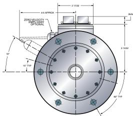
**Outline Dimensions (inch)** MCRT® **Maximum Overhung Moment** Model **Torque Range Spline Data** Dimension L ΑII 4,000 lbf-in 16 teeth, 20/30 D.P., 30° Pressure Angle 48850V 8 37/64 24 teeth, 20/30 D.P., 30° Pressure Angle 48851V All 4,000 lbf-in 9 5/64
