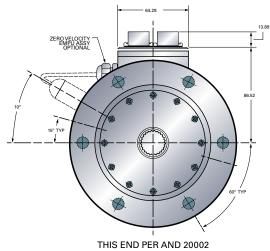
**Outline Dimensions (SI Units)** MCRT® **Maximum Overhung Moment** Dimension L Model **Torque Range Spline Data** All 16 teeth, 20/30 D.P., 30° Pressure Angle 48850V 452 N-m 218 ΑII 48851V 452 N-m 24 teeth, 20/30 D.P., 30° Pressure Angle 231
